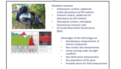
The AM350 measures an extended range of parameters. Real time image display, High resolution, Battery portable, Non-destructive, Fast and simple operation, Integral data and image storage, USB download of image and data
