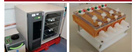
A climate controlled chamber and a drip flow bioreactor that will be used during the project to produce stable conditions during surface testing
